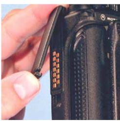
The universal connector cover protects the side connector near the antenna.
