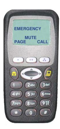
Note: To exit emergency at any time, press and hold the Emergency button for about a second.
