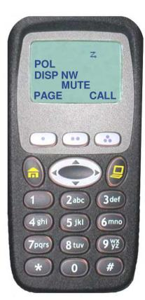
The scan feature allows you to monitor traffic on different channels by scanning a preprogrammed list of channels. Your radio can have several different scan lists. These lists must be preprogrammed by a qualified radio technician.
