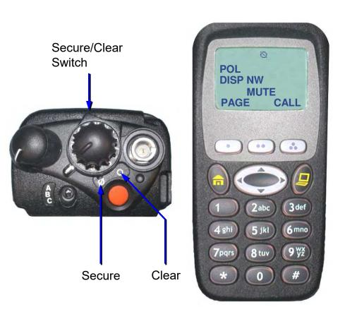
The radio will receive encrypted calls without enabling the Secure switch, but to transmit in secure, the Secure switch must be enabled.
