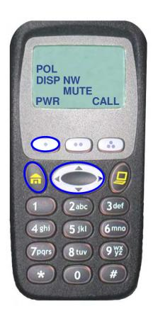
This feature lets you select the power level at which your radio will transmit. The radio will always turn on to the default setting. This feature must be preprogrammed by a qualified radio technician.
