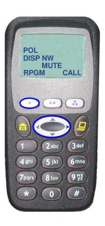
The dynamic regrouping feature lets the dispatcher temporarily reassign selected radios to a single special channel so they can communicate with each other.
