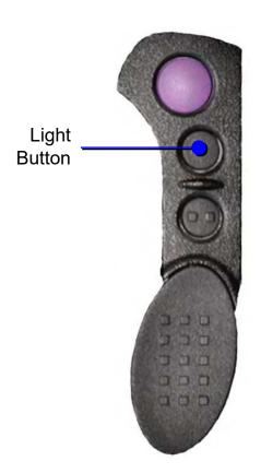
If poor light conditions make the display, keypad, or channel numbers (around the 16-Position Select knob) difficult to read:
