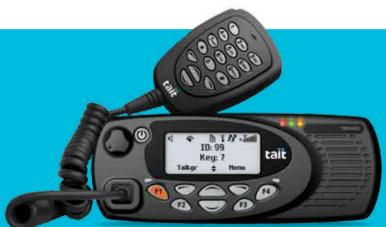
The TM9400 is capable of AES encryption, Over-the-air Rekeying (OTAR), various emergency modes and is IP54 rated to keep those relying on the mobiles safe and efficient. The TM9400 also has an options slot allowing extension of capabilities and a range of remote mounting and control head options.
